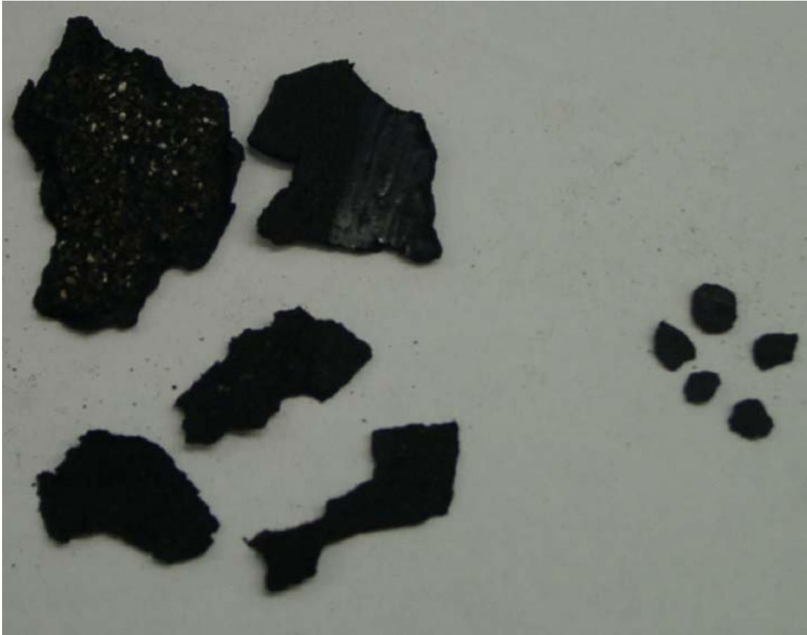
Figure 5.3 Photograph of RAS particles greater than 10 mm in size (left) and less than 10 mm in size (right)
