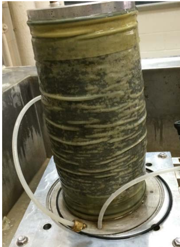
Figure 4.8. Axial bulging deformation in RAP specimen
