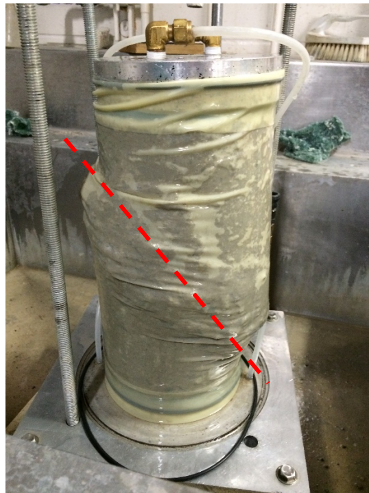
Figure 4.5. Failure plane for RCA specimens
