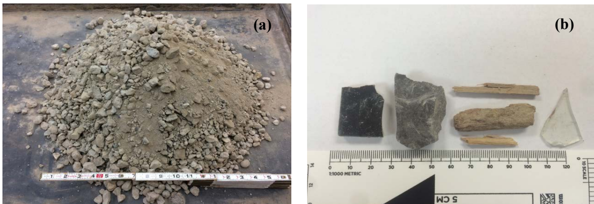
Figure 3.1. RCA sample from Mandt Sandfill, Fitchburg, WI (a) and impurities found in RCA sample include broken glass, wood, chips and tile pieces (b).
