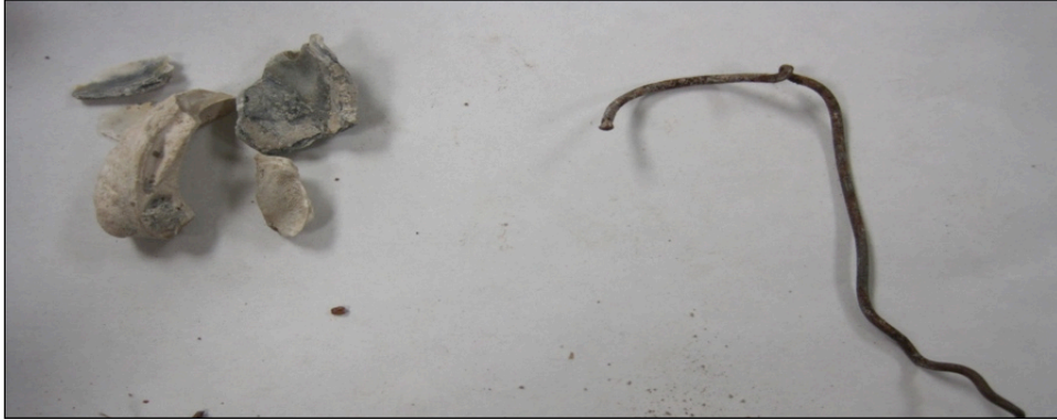
Fig. 6. Deleterious materials found in RCA: Sea shells and Steel
