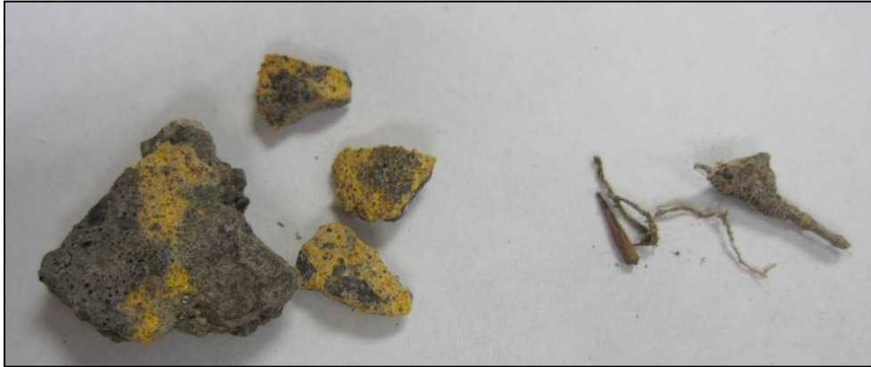
Fig. 8. Deleterious materials found in RAP: Pavement markings and wood chips
