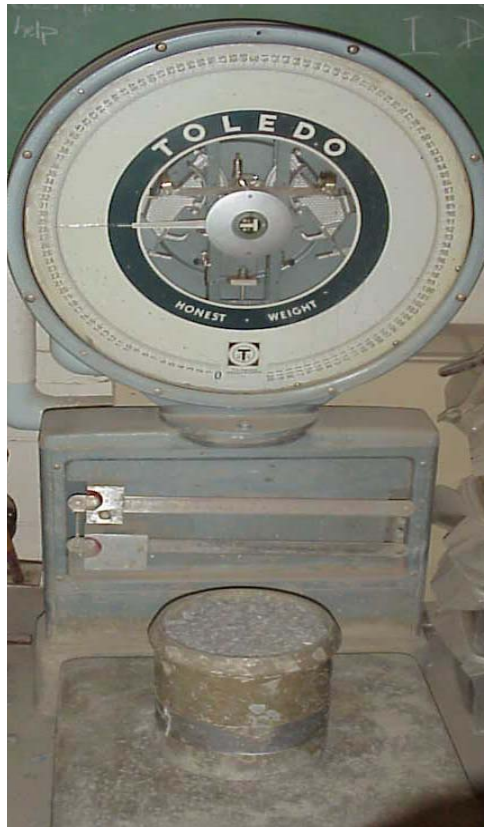
Figure 12 Steel bucket weighed
