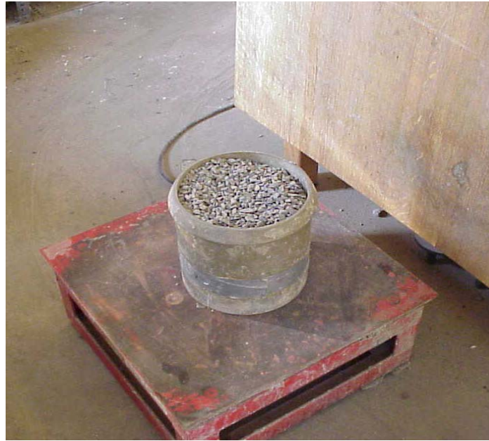
Figure 11 Steel bucket placed on vibrating table
