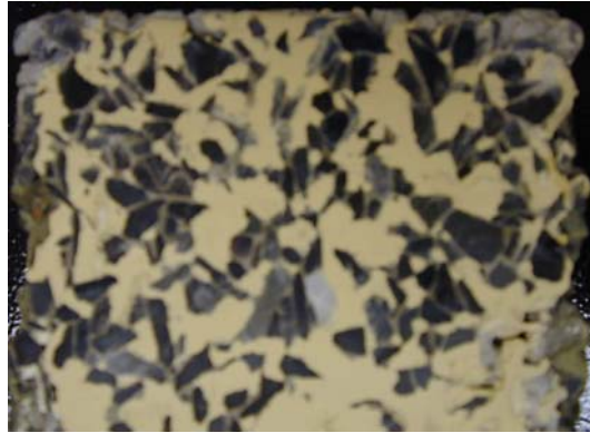
Figure 17 Concrete pores filled with Wood Putty®
