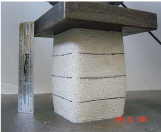
(b) Typical bulging failure has shown by extruded products from Mftg B and Mftg C.
