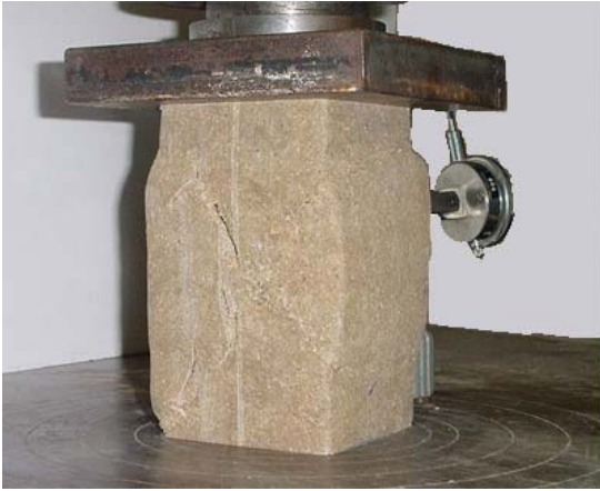
(a) Typical failure planes shown by compression molded RPPs from Mftg A.
