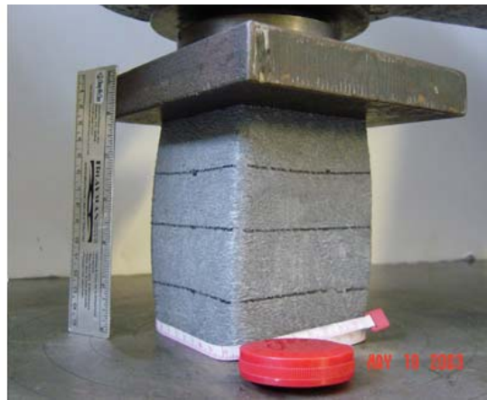
(b) Typical bulging failure has shown by extruded products from Mftg B and Mftg C.
