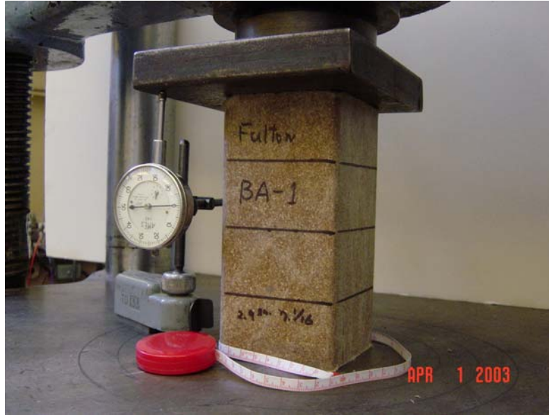
Figure 3.1 Setup for uniaxial compression tests.
