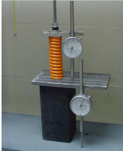
Figure 3.9 Setup for compressive creep test of recycled plastic specimen.
