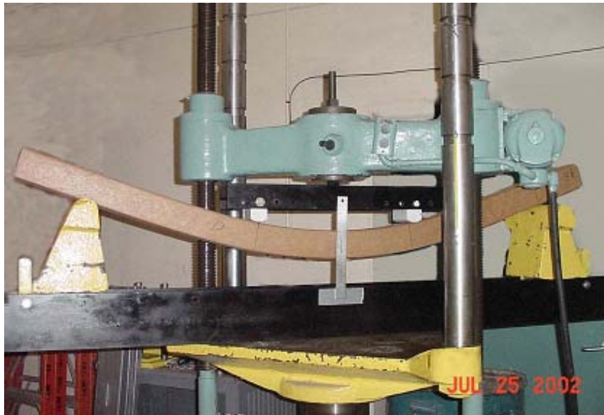
Figure 3.4 RPPs in the four-point flexure test.
