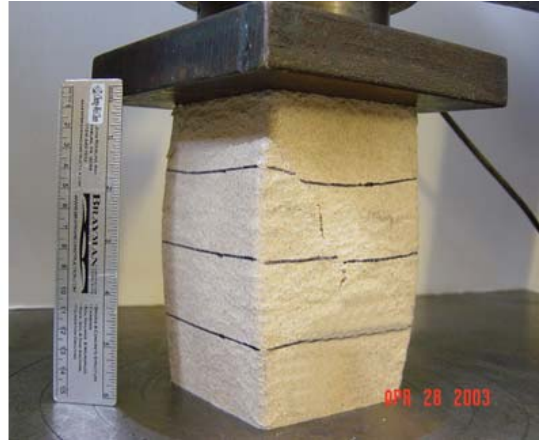
(a) Typical failure planes shown by compression molded RPPs from Mftg A.
