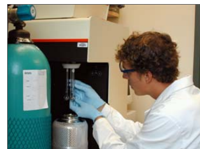
Graduate student Sandy Weymouth loads samples of steel slag into a Gas Adsorption Analyzer used to determine surface area.
