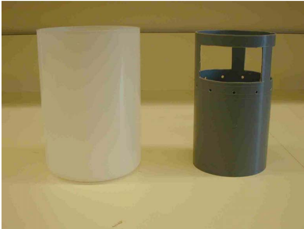
Figure 3.10. Compacted Granular Leaching Test mold (right) and leaching container (left).
