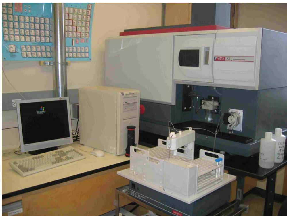
Figure 3.13. Varian ICP-AES used for inorganic analysis of leachates .
