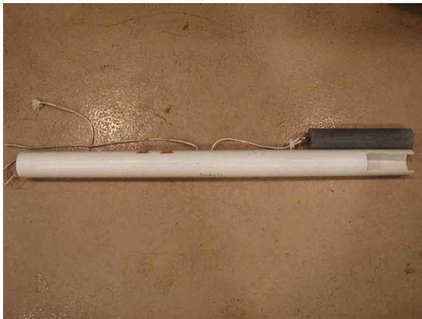
Figure 3.11. Ceramic hammer used for CGLT mold compaction.
