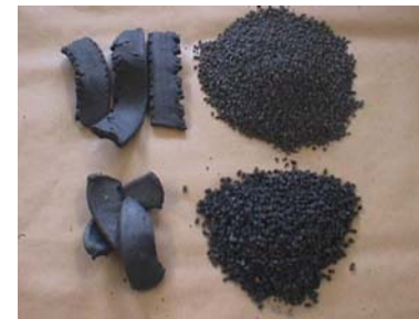
Extrudates on the left and granulated SLA on the right.
