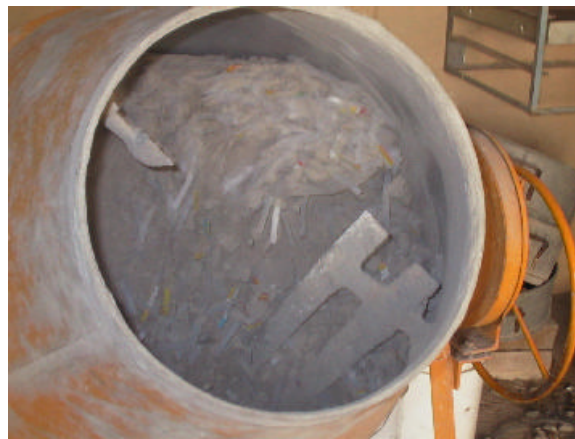
Figure 6. Materials were mixed in a rotary concrete mixer.
