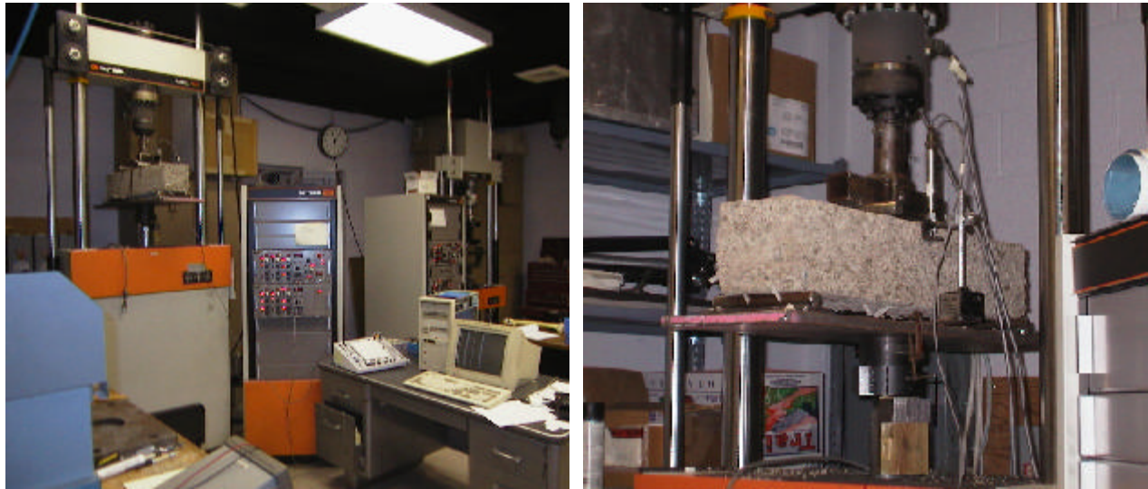
Figure 9. Instrument setup for flexural tests (left) and close-up of a beam and LVDT arrangements (right).
