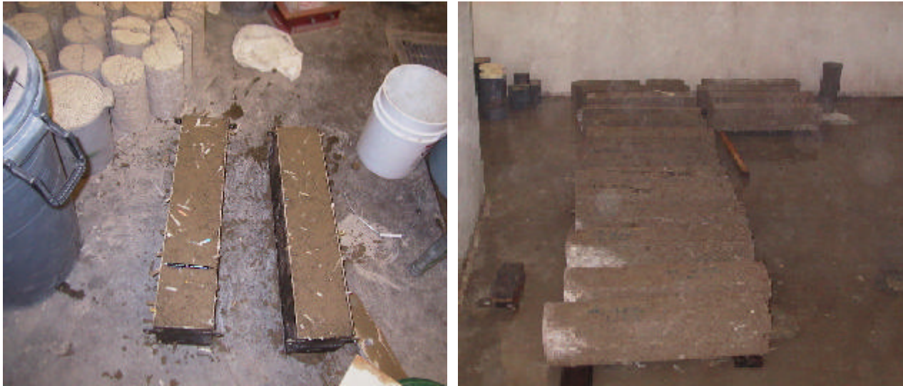
Figure 8. Preparation of beam specimens (left) and curing in humidity room (right).
