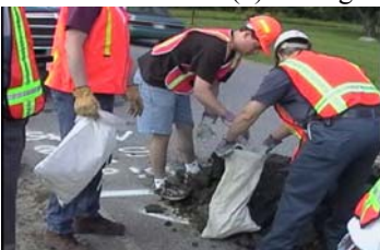
Figure 2. Sampling Existing Roadway Material
