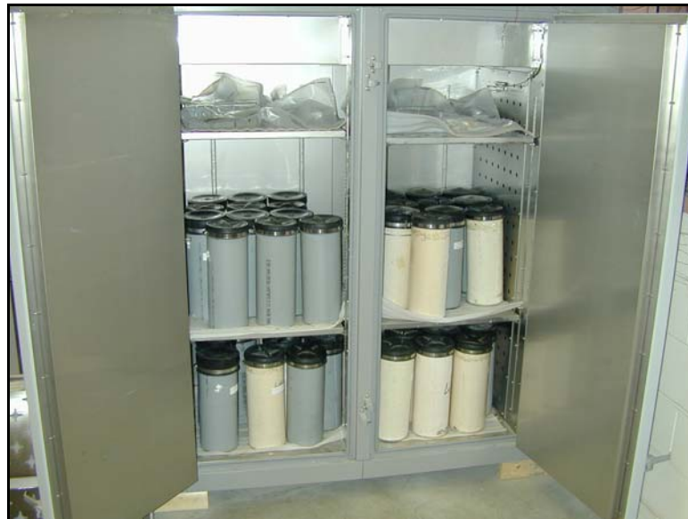
Figure 3-9: ASTM C 1293 Testing Oven
